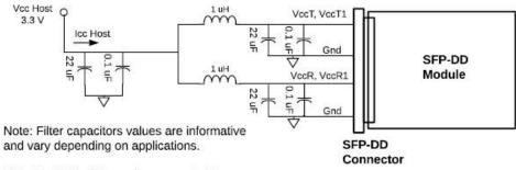
Note: VccT, VccT1 may be connected to VccR, VccR1 provided the applicable derating of the maximum current limit is used.
